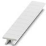
Zack marker strip, Strip, white, unlabeled, can be labeled with: PLOTMARK, CMS-P1-PLOTTER, mounting type: snap in, for terminal block width: 5.2 mm, lettering field size: 5.1 x 10.5 mm, Number of individual labels: 10
