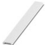
Zack Marker strip, flat, can be ordered: Strip, white, labeled according to customer specifications, mounting type: snap into flat marker groove, for terminal block width: 5 mm, lettering field size: 5.15 x 5.15 mm, Number of individual labels: 10
