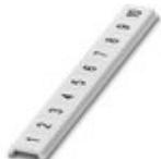
Zack Marker strip, flat, Strip, white, labeled, printed horizontally: consecutive numbers 1 ... 10, 11 ... 20, etc. up to 491 ... 500, mounting type: snap into flat marker groove, for terminal block width: 5 mm, lettering field size: 5.15 x 5.15 mm, Number of individual labels: 10
