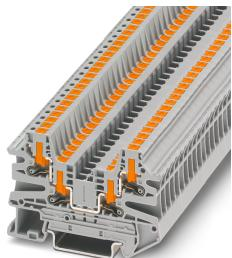
Feed-through terminal block, nom. voltage: 800 V, nominal current: 24 A, connection method: Push-in connection, 1 level, Rated cross section: 2.5 mm<sup>2</sup>, cross section: 0.14 mm<sup>2</sup> - 4 mm<sup>2</sup>, mounting type: NS 35/7,5, NS 35/15, color: gray
